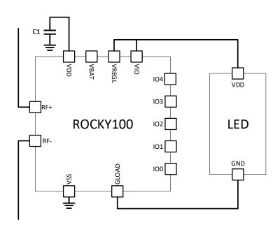
The ROCKY100 IC includes the RF frontend for UHF RFID power harvesting and communication, a power supply module to generate the required voltage levels, and an EPC C1G2/ISO18000-6C digital processor including a PWM module.
